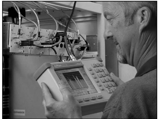
Figure 5. Cell Master measures the cdma2000 1xEV-DO signal by connecting to the base station.
