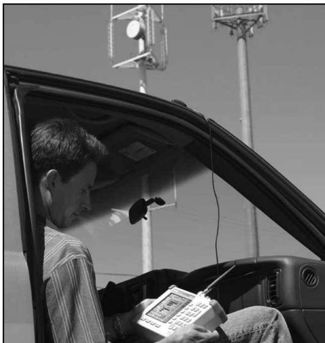
Figure 6. Cell Master can also demodulate the 1xEV-DO signal using an over the air antenna. A built-in GPS feature provides users with UTC time and location information.
